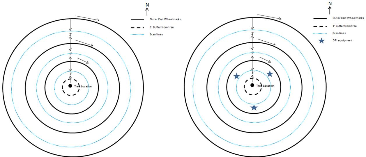
Figure 26: Scan layout for trees with surface drip irrigation (left) and DRI (right) system
