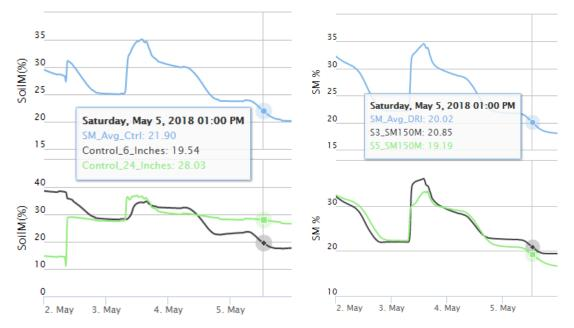
Figure 14: Soil moisture level at the DRI (right) and control (left) trees on May 05, 2018 at 1 p.m.
