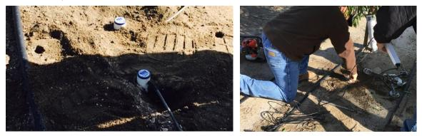
Figure 9: SENTEK soil moisture probe installation
