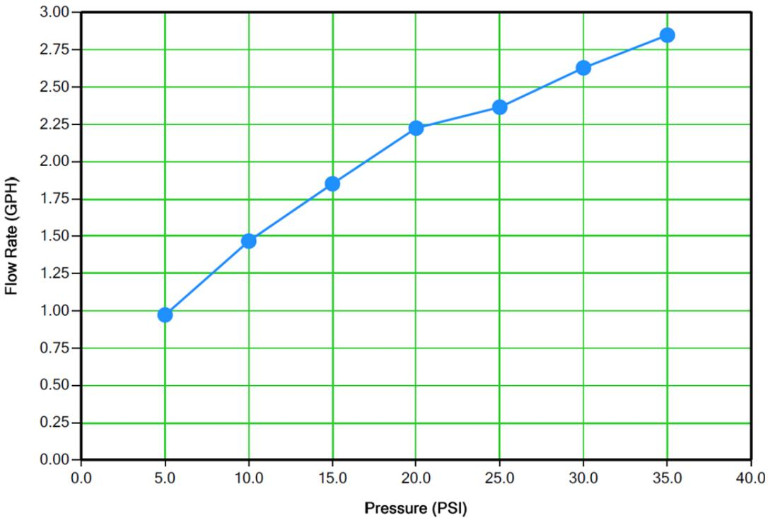
The flow rate of the drip emitters and DRI units attached with them in the field was tested next by collecting field data and the results are represented below.
