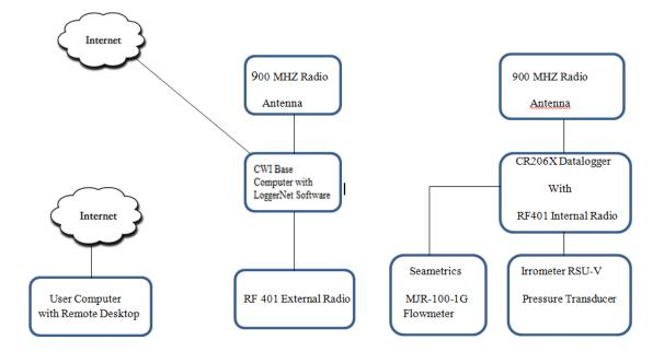
Figure 11: Flow diagram of system design
