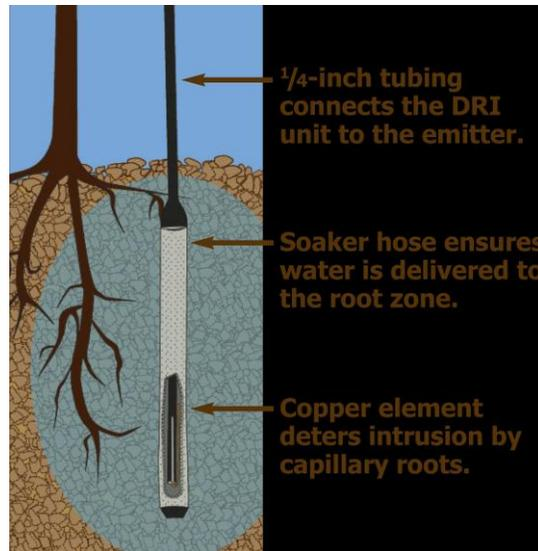
Figure 7: DRI equipment design as inserted underground
