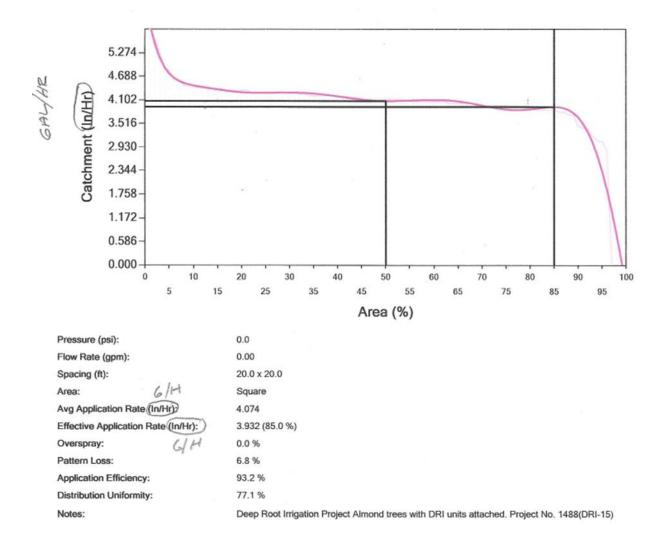
Figure 45: Irrigation water distribution uniformity test result
