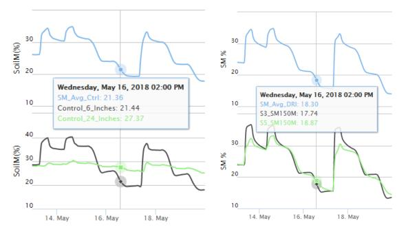
Figure 16: Soil moisture level at the DRI (right) and control (left) trees on May 16, 2018 at 2 p.m.
