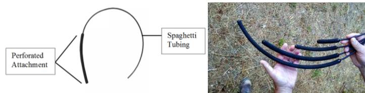
Figure 6: DRI equipment with two parts (left), and different sizes (right)
